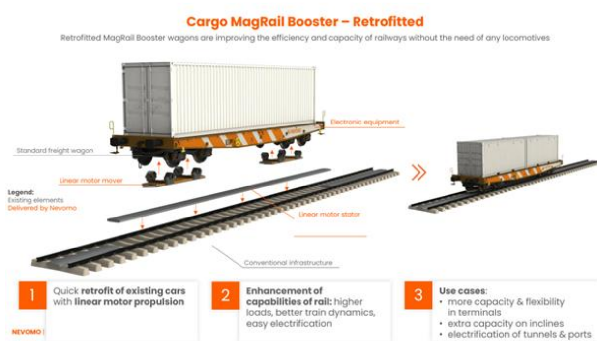
Figure 3.2. Cargo MagRail Booster, retrofit
